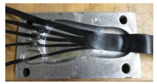
Figure 21 71 cm piece aligned in mold.
