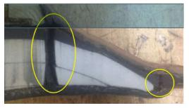
Figure 1 Gaps due to shrinkage of the EVA blocks.
