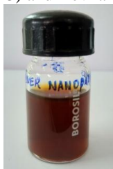
Fig. 1 Color change after the process of bio-reduction of silver-to-silver nanoparticles
