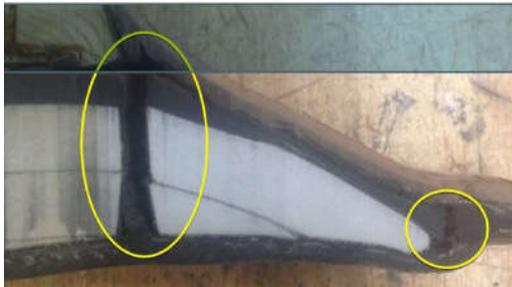
Figure 1 Gaps due to shrinkage of the EVA blocks.
