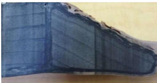
Figure 2 Gaps were eliminated by using Nylon 6 that shows no shrinkage.
