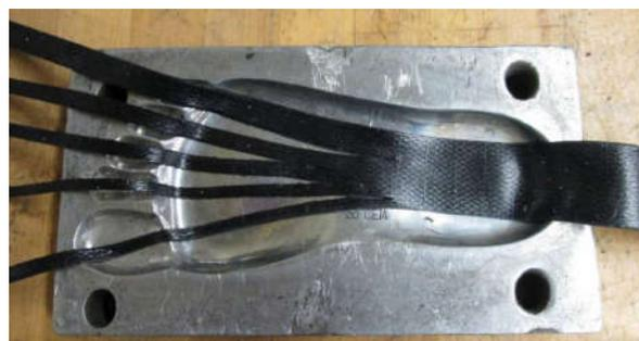
Figure 21 71 cm piece aligned in mold.
