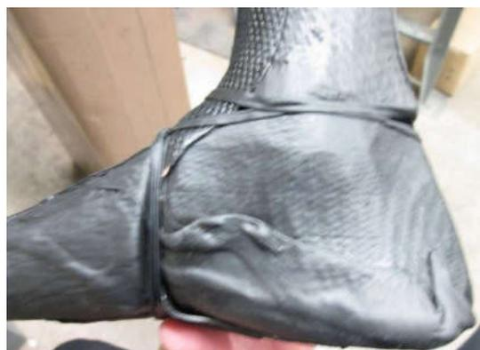
Figure 20 Cushion compound between Forefoot, heel and ankle blocks.
