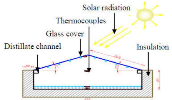
Figure 2 Schematic diagram of the double slope solar still
