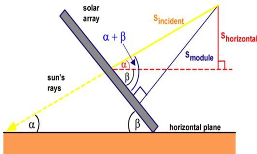
Figure 1 Tilting the module to the incoming light reduces the module output
