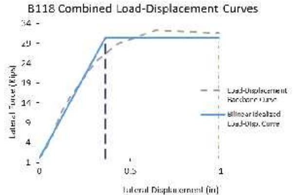
Figure 4 Actual and Idealized Load-Deflection curves of Sample-B118 (1900 psi, 5in c/c)
