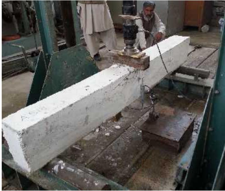
Figure 2 Setup for testing of beams with Displacement Gauges and Load Cell installed at straining frame assembly
