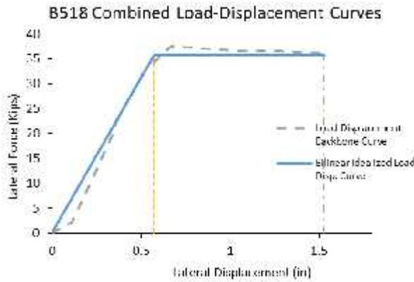
Figure 6 Actual and Idealized Load-Deflection curves for Sample-B518 (1800psi, 2.5in c/c, Extra Negative Reinforcement)
