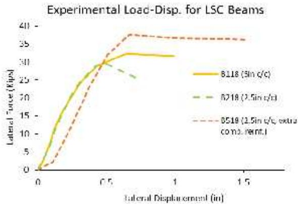
Figure 3 combined experiments load-deflection curves for 1900 psi beams
