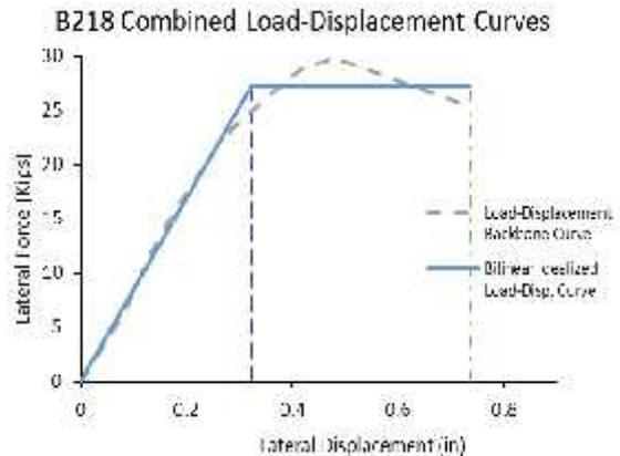
Figure 5 Actual and Idealized Load-Deflection curves of Sample-B218 (1900 psi, 2.5in c/c)
